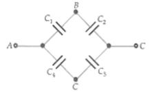
Capacitors C<sub>1</sub> and C<sub>2</sub> form a series combination of equivalent capacitance C<sub>6</sub> given by
