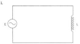
Induced emf,  $e = -L\frac{dI}{dt}$ Hence, Net voltage in the circuit  $= V - L\frac{dl}{dt}$ According to Kirchhoff s Rule  $V - L\frac{dI}{dt} = 0$   $V_m \sin \omega t = L\frac{dI}{dt}$   $dI = \frac{V_m}{L} \sin \omega t dt$   $I = -\frac{V_m}{\omega L} \cos \omega t$   $= \frac{V_m}{\omega L} \sin (\omega t - \frac{\pi}{2})$   $\therefore I = I_m \sin (\omega t - \frac{\pi}{2})$ Hence current lags by  $\frac{\pi}{2}$
