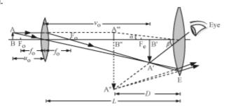
where AB = object, A'B' = image formed by objective, A''B'' = image formed by eyepiece L is the separation between the eyepiece and the objective,
