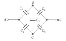
As  $C_1 = C_2 = C_4 = C_5$ Therefore,  $\frac{C_1}{C_2} = \frac{C_4}{C_5}$
