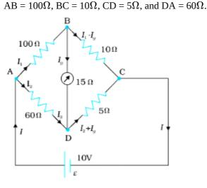
A galvanometer of  $15\Omega$  resistance is connected across BD. Calculate the current through the galvanometer when a potential difference of 10 V is maintained across AC.
